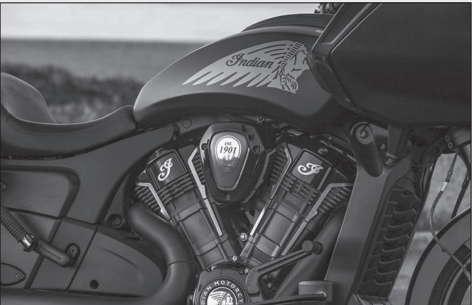
The heart of the Challenger is Indian Motorcycle’s 107ci (1,768cc) PowerPlus V-twin engine. This twin is good for 103 hp and nearly 114 pound-feet torque at the business end of the Metzeler back tire.
