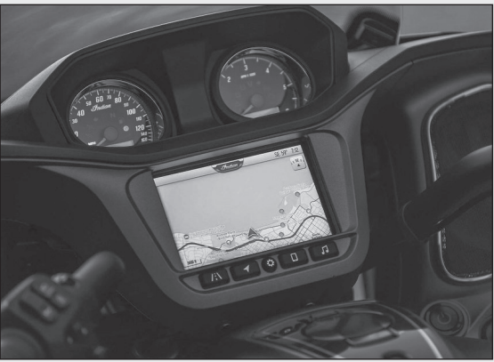
Indian Motorcycle’s Ride Command 7-inch touchscreen display works well. Its menu system is logical, and it’s loaded with a rich amount of features including trip analytics and the ability to pair a Bluetooth-enabled smartphone. The Dark Horse edition adds GPS navigation and IMU-powered traction control.)
