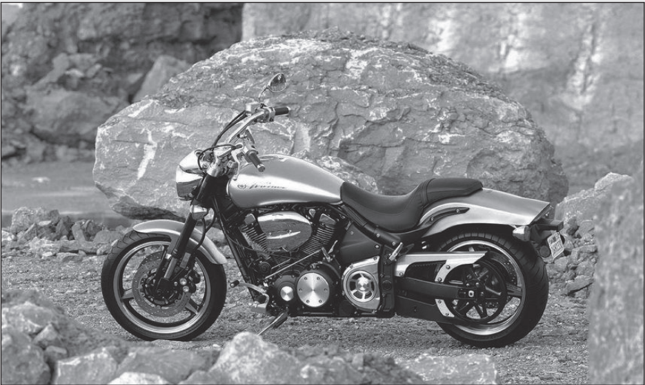
The Road Star Warrior remains desirable today for its aluminum chassis, hot-rod air-cooled motor, and sportbike suspension and brakes.
