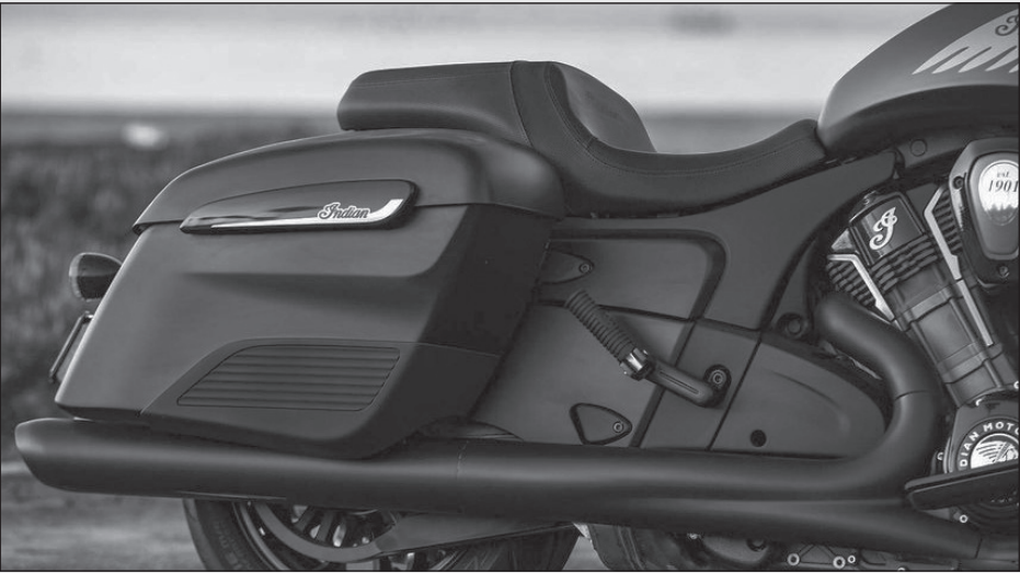
The Challenger comes outfitted with a pair of electronically lockable hard cases that are capable of swallowing up to 18 gallons of gear. The bags aren’t wide enough to accommodate a full-face helmet.
