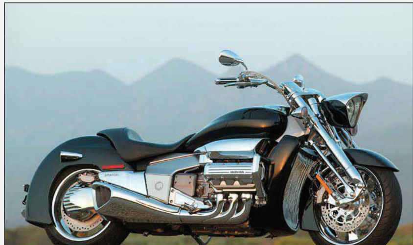
The wildest of all Valkyries was the limited-production Rune, produced in 2004 and 2005. Dual 330mm front and single rear 336mm brake discs were also the largest ever fitted to a production Honda.
